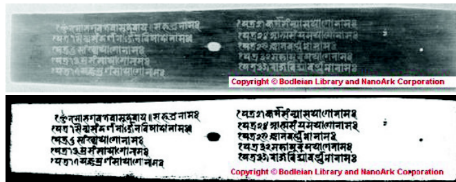
(Top): Scanned image of palm leaf with illegible text due to low contrast. (Bottom): Restored image of palm leaf with discernable text.
